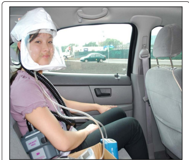
Figure 3 An investigator demonstrates set-up of the powered air purifying respirator, with sampling instrument inlets in place inside the respirator facepiece, as worn by subjects.
