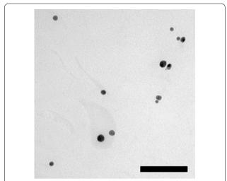
**Fig. 1** Transmission electron micrograph of PVP-coated silver nanoparticles in ultrapure water. The scale bar is 100 nm
